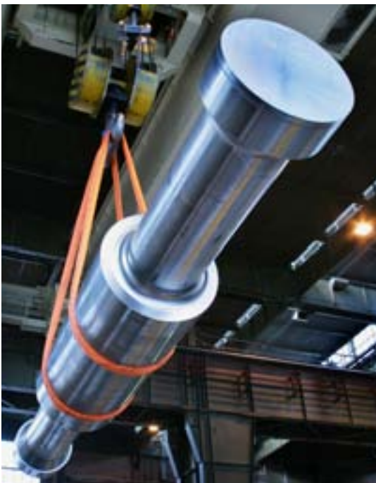
MD-Turbinenwelle MP Turbine Shaft
