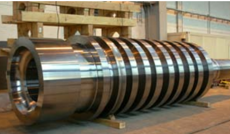
MD-Turbinenwelle MP Turbine Shaft
