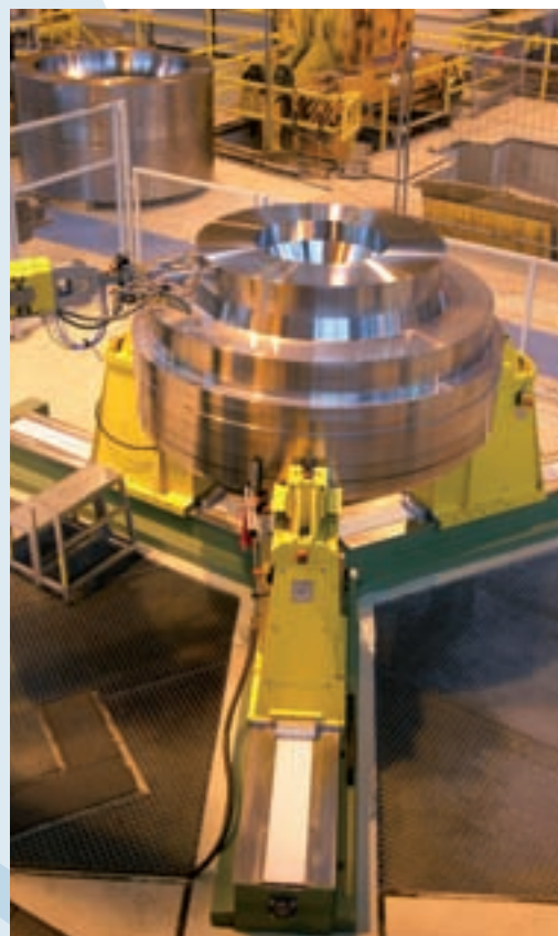
Ultraschall-Scheibenprüfanlage Ultrasonic Testing Facility for Discs
