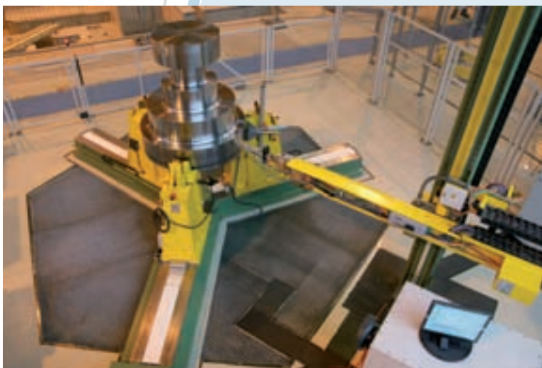
Ultraschall-Scheibenprüfanlage Ultrasonic Testing Facility for Discs
