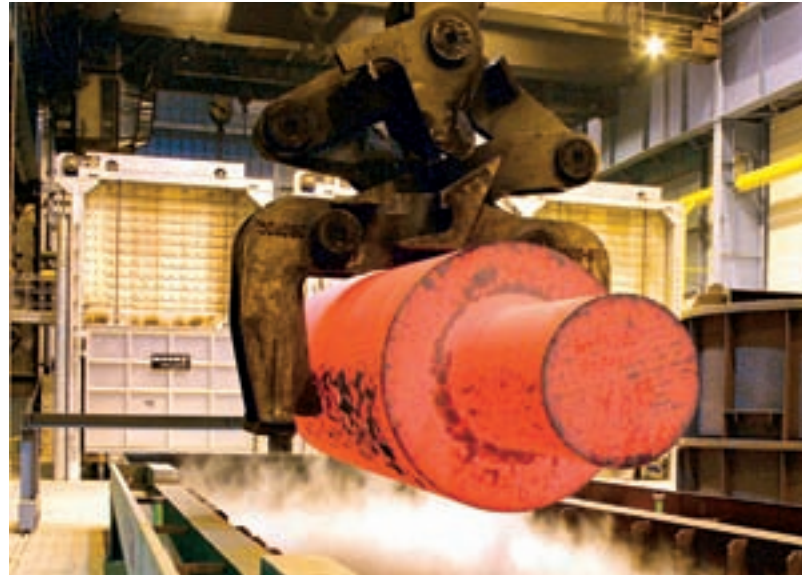
ND-Welle beim Härten | Low Pressure Turbine Shaft during Hardening
