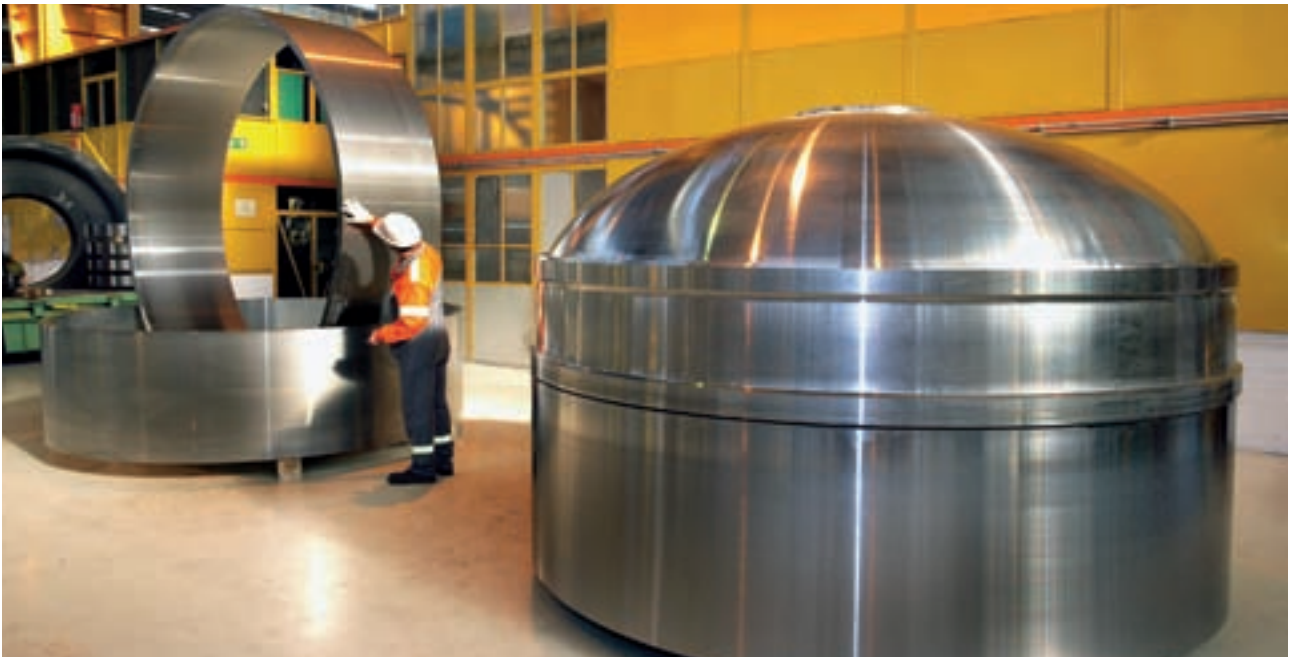
ARIANE 5 Ringe und Dom, LBO-VL-1.6944X2 (D6AC) ARIANE 5 rings and dome, EAF-VAR-1.6944X2 (D6AC)
