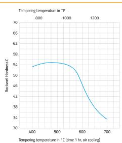
Tempering temperature in  $^{\circ}$ C (time 1 hr, air cooling) Quenched from 1010 $^{\circ}$ C / 1850 $^{\circ}$ F in oil Average values obtained on Ø 25 x 50 mm long samples
